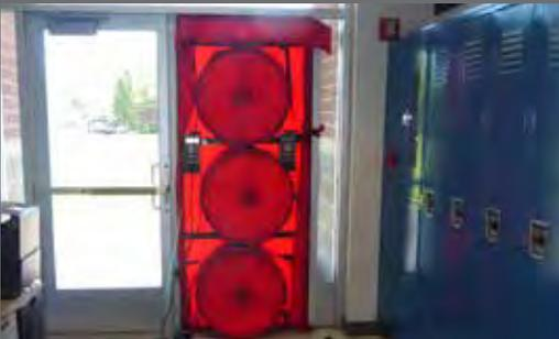
Air Barrier Solutions conducted blower door testing pre-and post-retrofit to measure air tightness. Prior to retrofitting, the building air leakage was severe resulting in moisture problems, comfort issues, and significant energy losses. CcSPF was used to improve air tightness exceeding the International Green Construction Code requirements.
