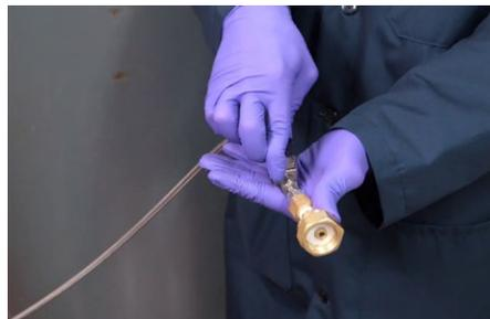
2. Before connecting the nitrogen gas hose to the blowing agent cylinder vapor port, check again that the CGA-660 connection has the required gasket.
