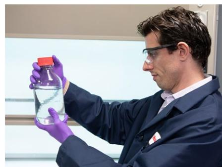
Image shows Solstice LBA being dispensed into an open container. NOTE: Solstice GBA **MUST** be dispensed into an appropriate pressure-rated container or process line of a closed system.
