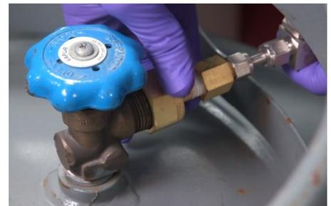
3. Remove the cap from the blue vapor port, which will be used for the nitrogen vapor to enter the blowing agent cylinder. Connect the nitrogen gas hose to the blue vapor port and secure tightly.
