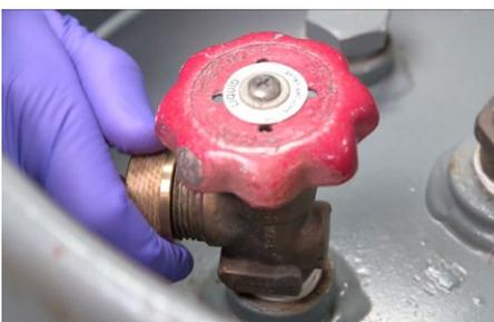
4. The final step is to connect the liquid discharge line. Remove the cap from the red liquid discharge port on the blowing agent cylinder. Before attaching the liquid discharge line to the port on the blowing agent cylinder, make sure to check for the required gasket. It is also critical to ensure that the line is rated for the desired pressure and the hose material is compatible with the blowing agent.
