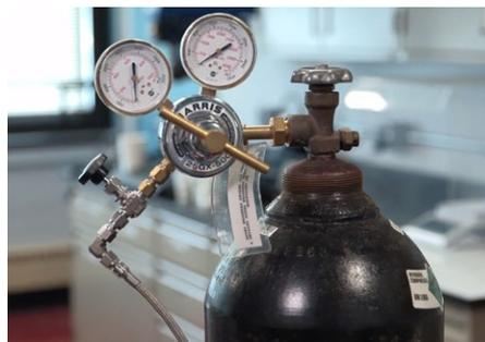
A two-stage nitrogen regulator is required.
