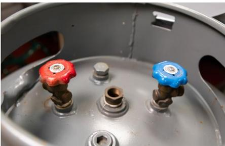
1. To prepare the 1,000 lb. (454kg) half-ton cylinder for pressurization, start by lifting the cap. This should reveal two handles and two ports on the cylinder's top.
