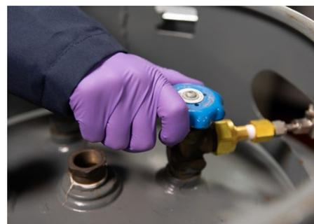
4. Finally, open the vapor valve on the blowing agent cylinder to allow the nitrogen gas to flow into the cylinder, pressurizing it.
