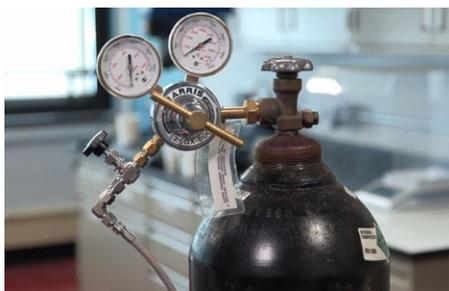
1. With the lines connected, the blowing agent cylinder can be pressurized. This is done by turning the handle on the top of the nitrogen cylinder to the open position and adjusting the regulator to dispense the nitrogen gas at a pressure of 100 psi (690 kPa). Remember not to exceed this pressure.
