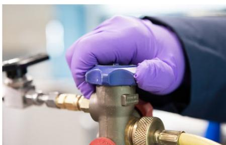
4. Finally, open the vapor valve on the blowing agent cylinder to allow the nitrogen gas to flow into the cylinder, pressurizing it.
