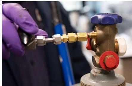
2. This should reveal two handles and two ports at the top of the cylinder. Remove the cover from the smaller port, which will be used for the nitrogen gas to enter the blowing agent cylinder.
