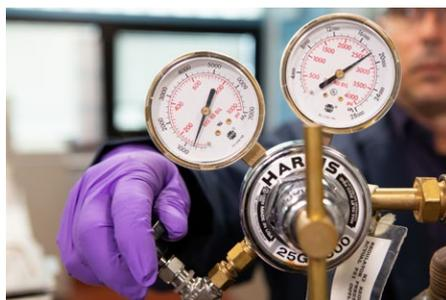
2. You can then open the needle valve at the nitrogen regulator to start the flow of nitrogen.
