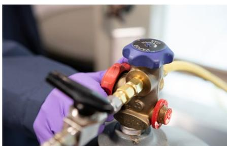
4. If both these requirements are met, connect the liquid discharge line and secure tightly.
