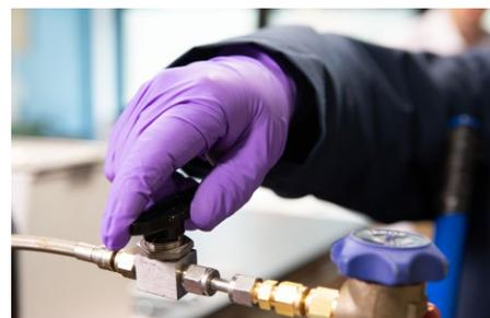
3. Next, open the valve on the nitrogen line near the blowing agent cylinder.
