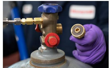
3. Next, remove the cap from the larger liquid discharge port on the blowing agent cylinder.
