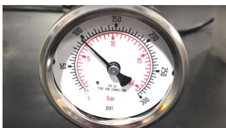
Be sure that your nitrogen regulator can be set to 100 psi (690 kPa).
