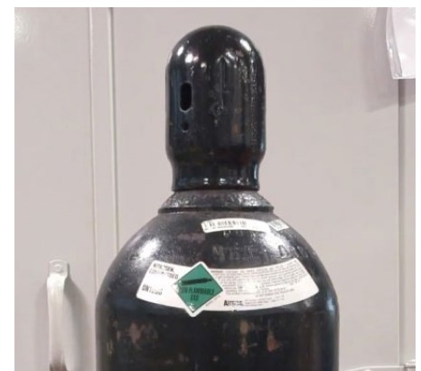
If in-house nitrogen is unavailable, 100 lb. (45.4 kg) nitrogen cylinders can be used.
