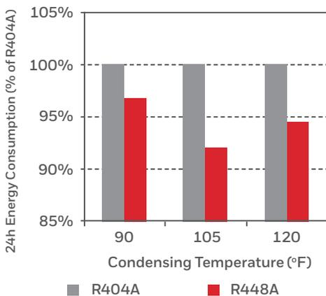
Left: In recent laboratory tests at Emerson Climate Technologies, Solstice N40 demonstrated up to 8% lower energy consumption than R404A.
