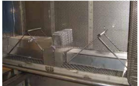
Basket of Parts in Post-Degreasing Process
